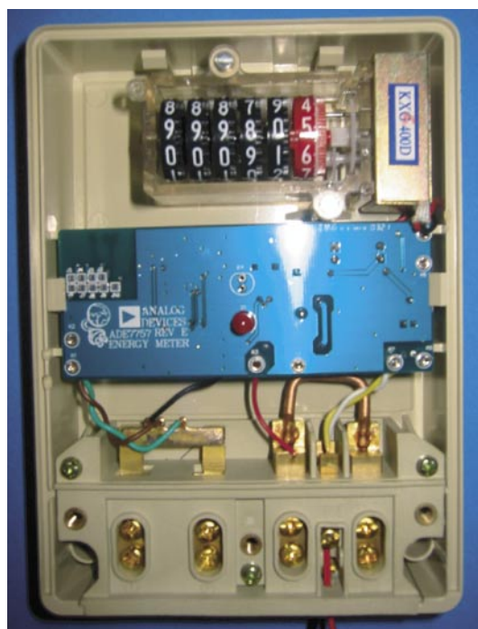
Figure 2. Final Implementation of ADE7757 Meter
